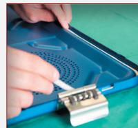
Accurate gluing of the silicone seal into the container lid
