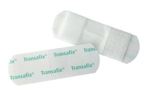
The lead or probe can either move freely within the Velcro strap or be fixed securely by taking of the protective cover, uncovering an adhesive film. The Velcro strap can be opened and closed as often as you like. Hence, the fastening strip doesn't have to be removed when exchanging the probe.
