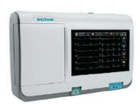
This is a new generation 3-channel ECG, which incorporates benefits of the advanced technology and innovative design. The device has an extremely compact and lightweight body and is designed for emergency rooms, home visits, etc.
