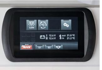
Many central functions such as lighting or air conditioning and heating systems can be controlled via the touch panel in the patient compartment.
